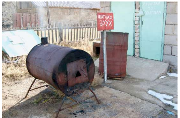
Hospital's medical waste burning container
